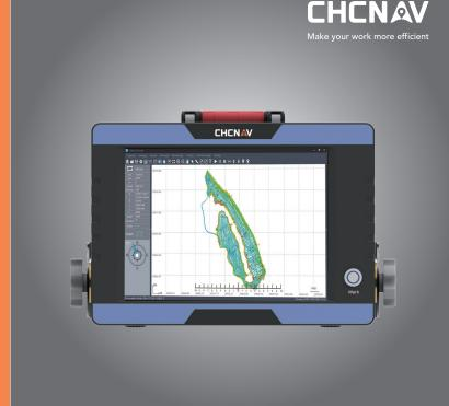
D580 is a revolutionary dual-frequency echo sounder which has 200 kHz and 25 kHz as high and low frequency. The integration design and light weight (less than 6 kg) can make it easy to carry. Meanwhile, D580 develops superior functions such as showing real-time depth graph with high or low frequency respectively and adopting integrated transducer, etc.
